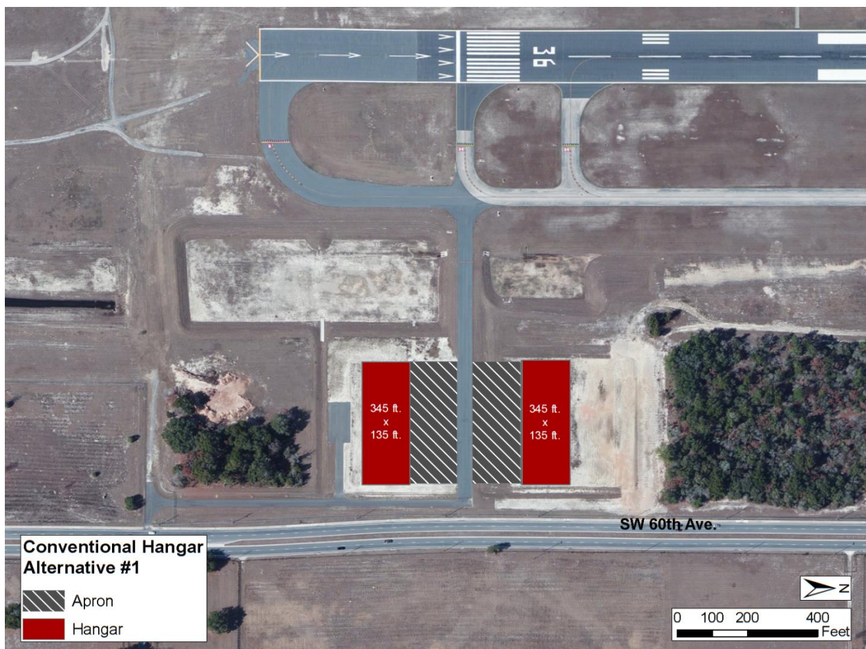
Exhibit 6-18 Conventional Hangar Alternative #1
