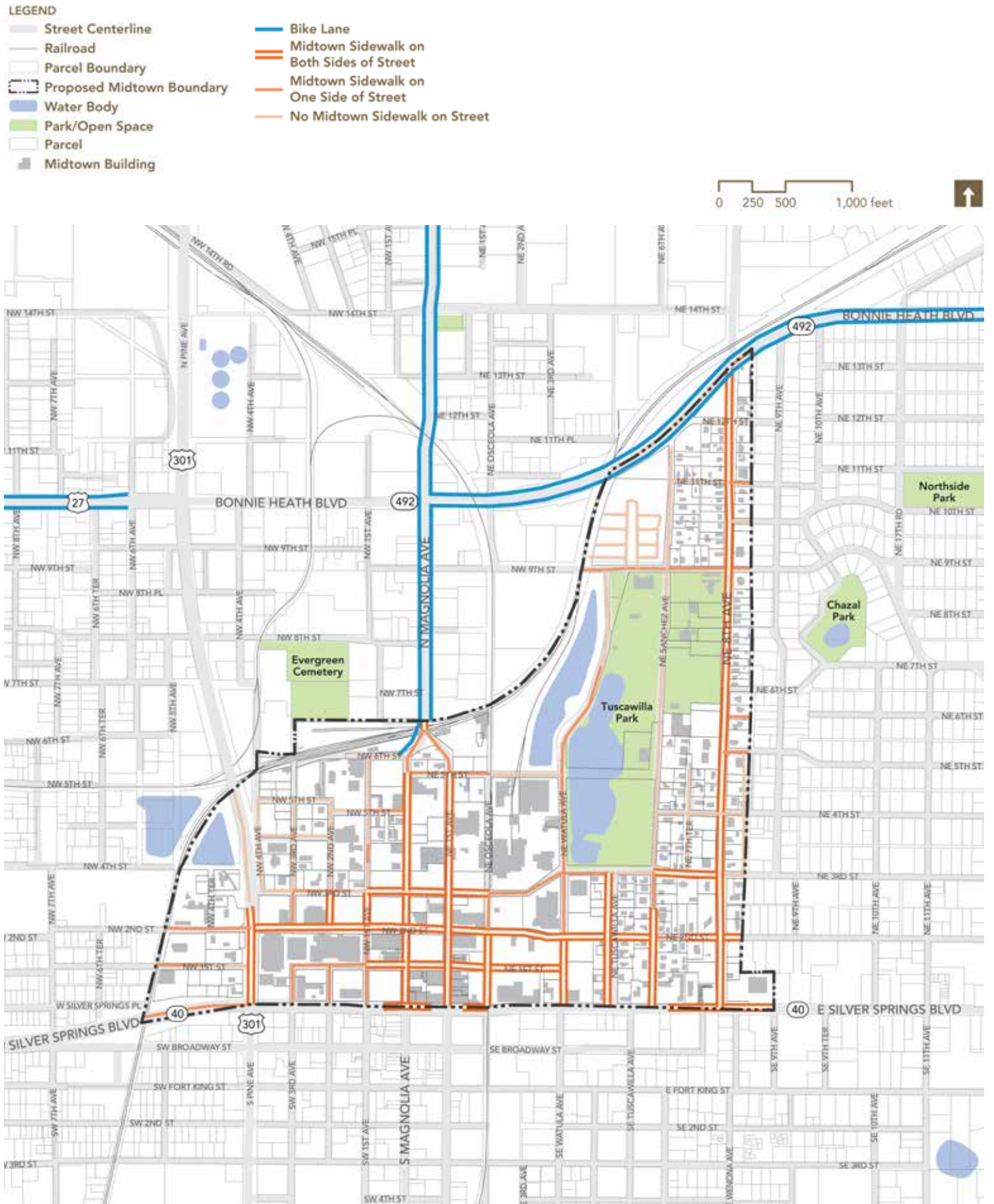
Figure 2.5: Pedestrian and Bicycle Facilities
